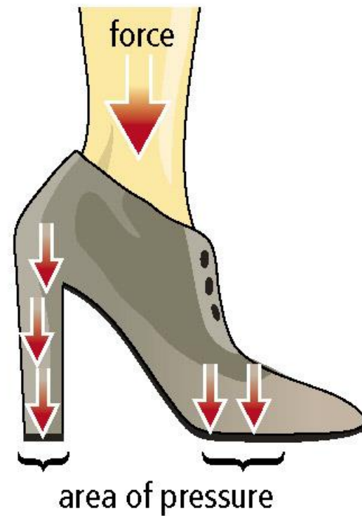
Figure 9.14A and 9.14B High heels exert more pressure on the ground because the pressure is concentrated into a smaller area than a flat shoe.
